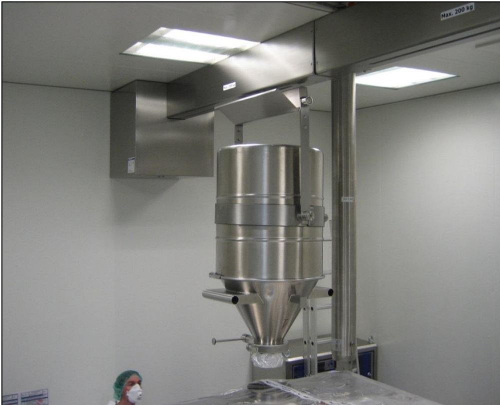
Monorail twin-crane for two-sided feeding of a pill press.
